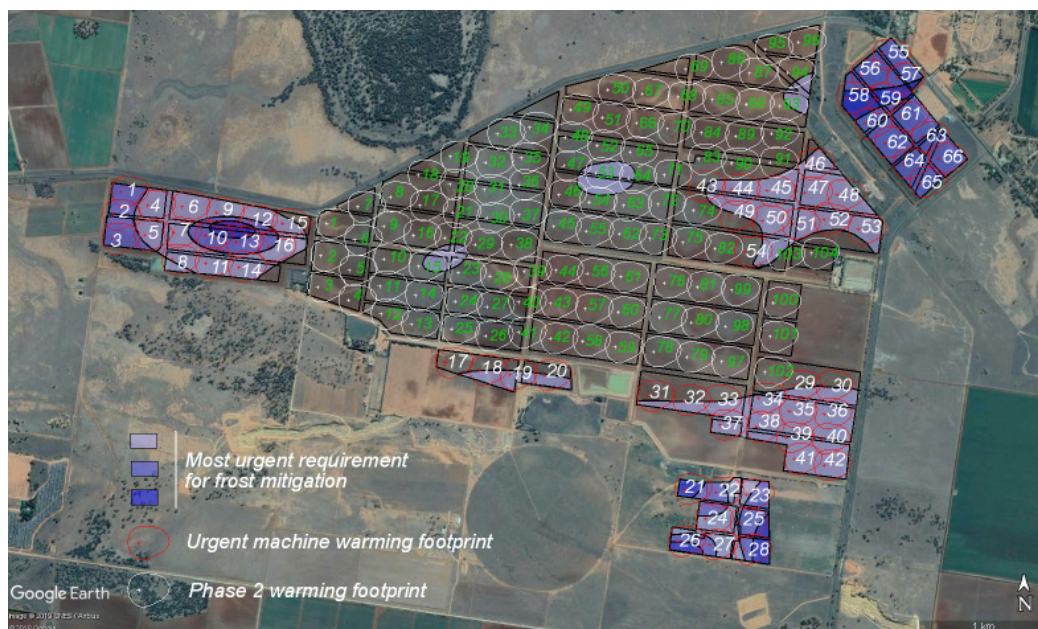
Figure 14b A further 104 wind machines would be necessary to protect remaining areas of the orchard. Final wind machine numbers will reflect machine make and model.
